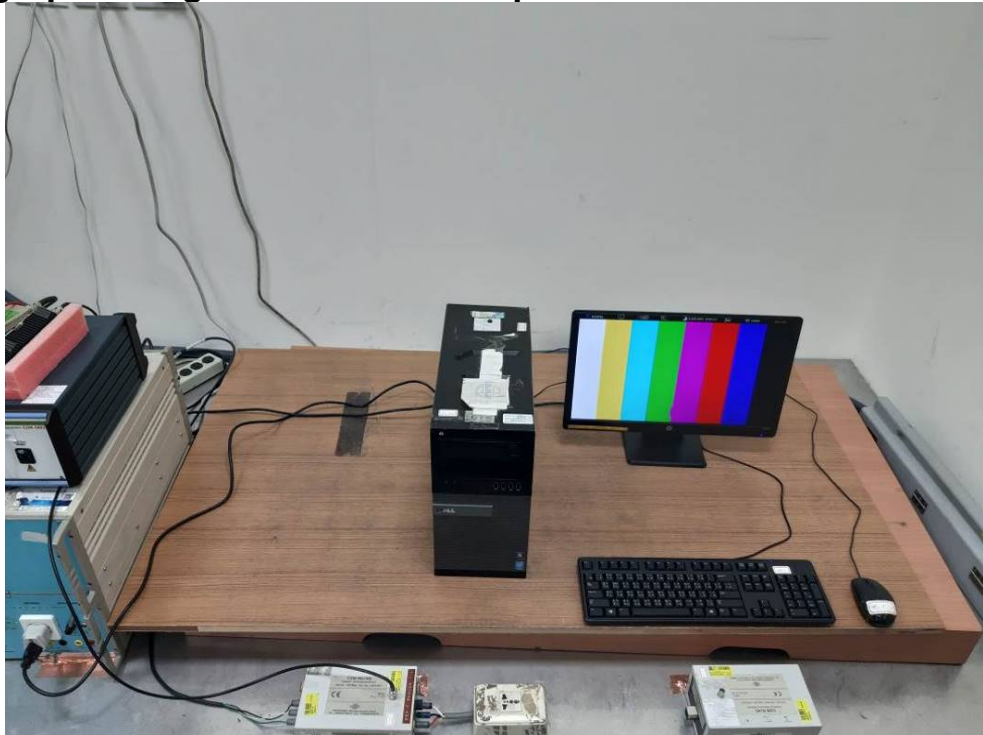
Photograph –Surge & EFT Test Setup
