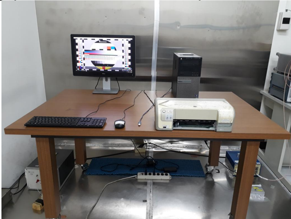
Photograph – Conducted Emission Test Setup
