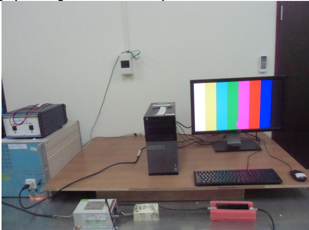
Photograph –Surge & EFT Test Setup
