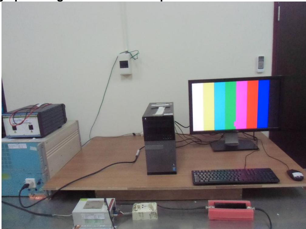
Photograph –Surge & EFT Test Setup
