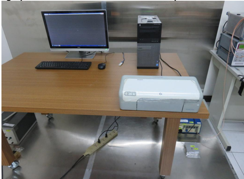
Photograph – Conducted Emission Test Setup
