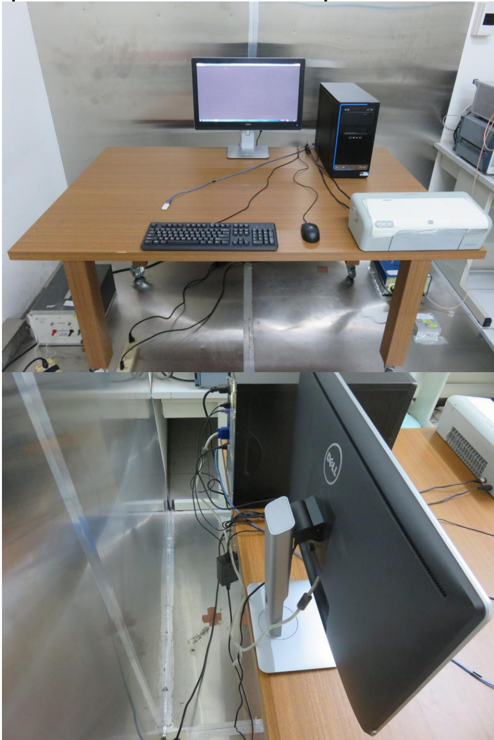
Photograph – Conducted Emission Test Setup
