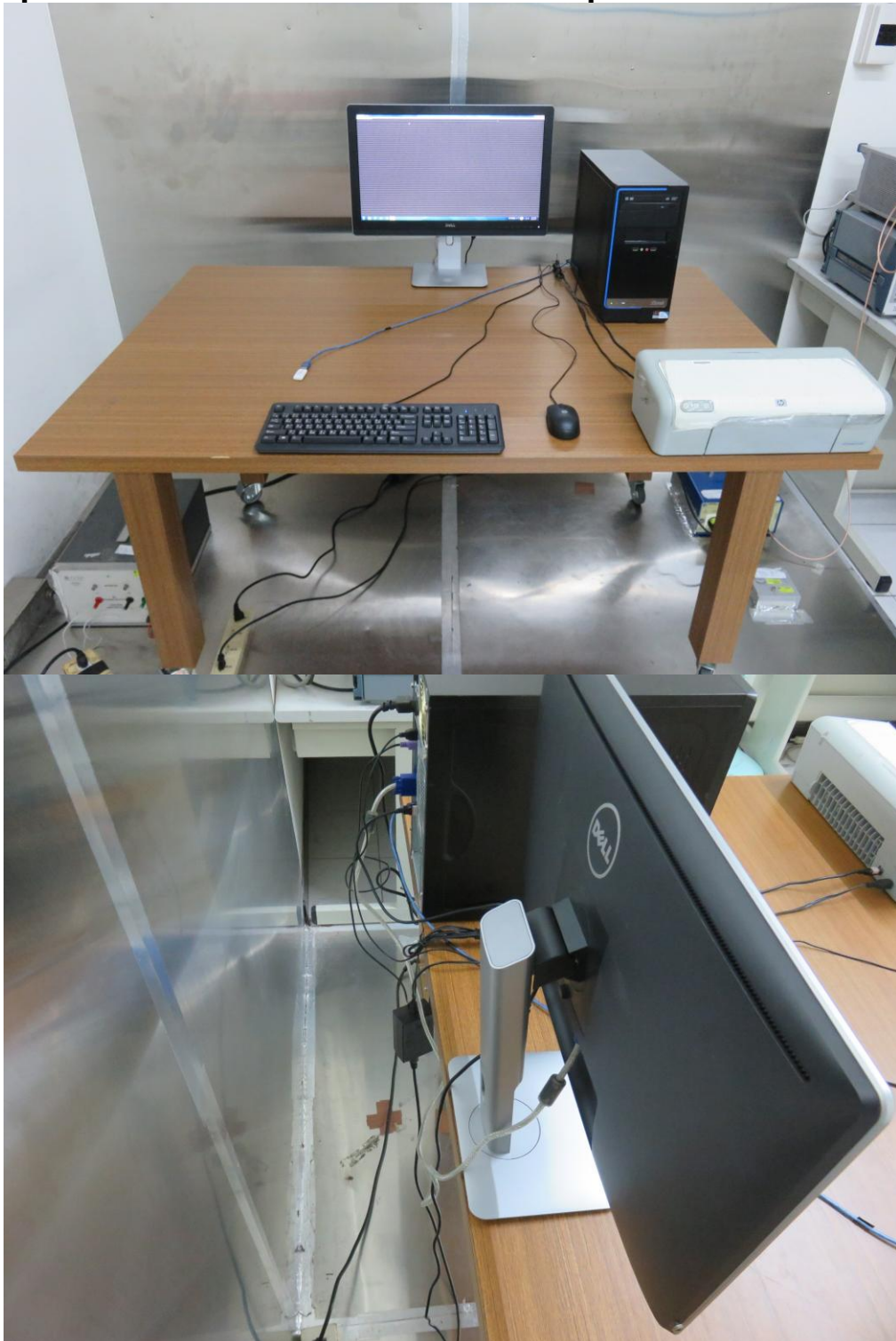
Photograph – Conducted Emission Test Setup
