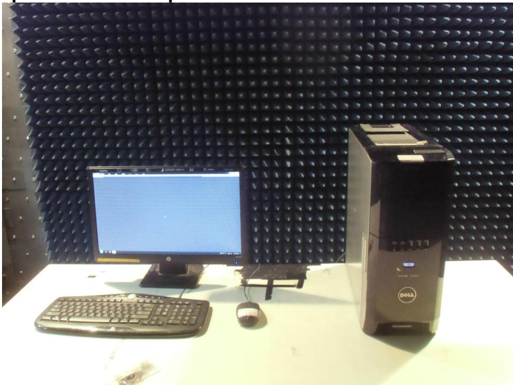
Photograph –RS Test Setup
