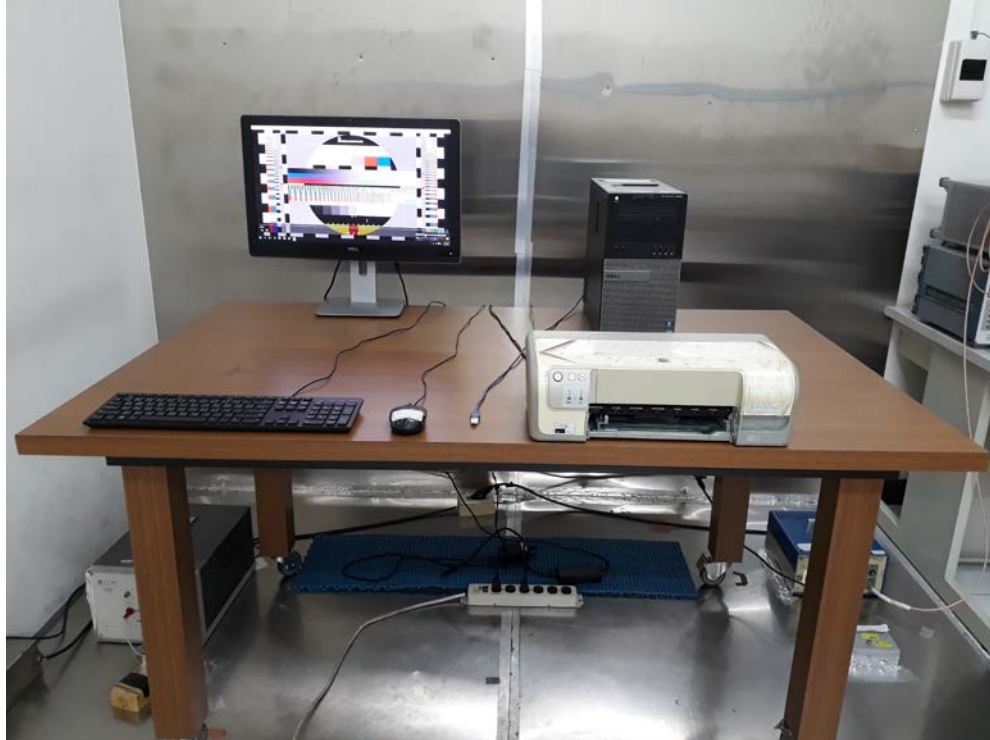
Photograph – Conducted Emission Test Setup
