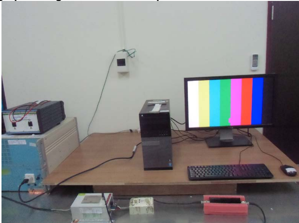
Photograph –Surge & EFT Test Setup
