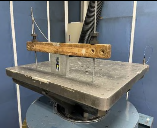
16. Non-Operating Vibration Test (Y axis)
