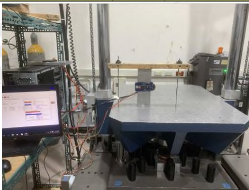
11. Operating Mechanical Shock Test (+Y axis)
