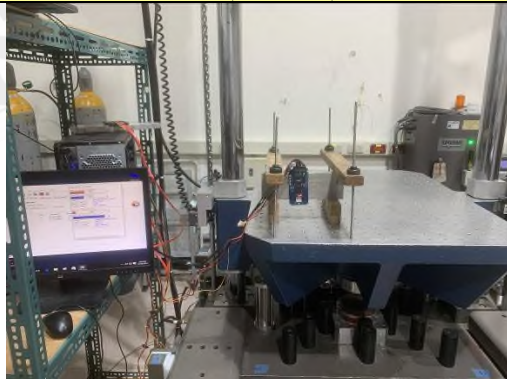
9. Operating Mechanical Shock Test (+X axis)
