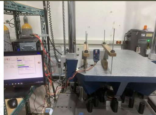
10. Operating Mechanical Shock Test (-X axis)
